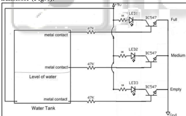
Fig. 4: Level sensor setup
