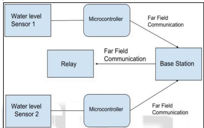
Fig. 1: Schematic of single node
