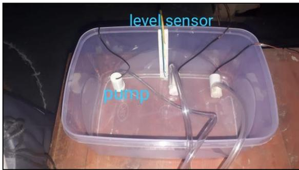
Fig. 5: water tank with level sensors and pumps
