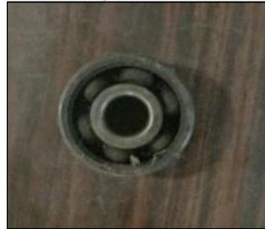
Fig. 7.8: Ball Bearing
