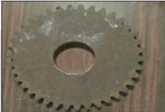
Fig. 7.6: Spur Gear
