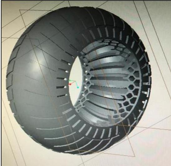
Fig. 11: 3-D Airless tire design (Version-G)
