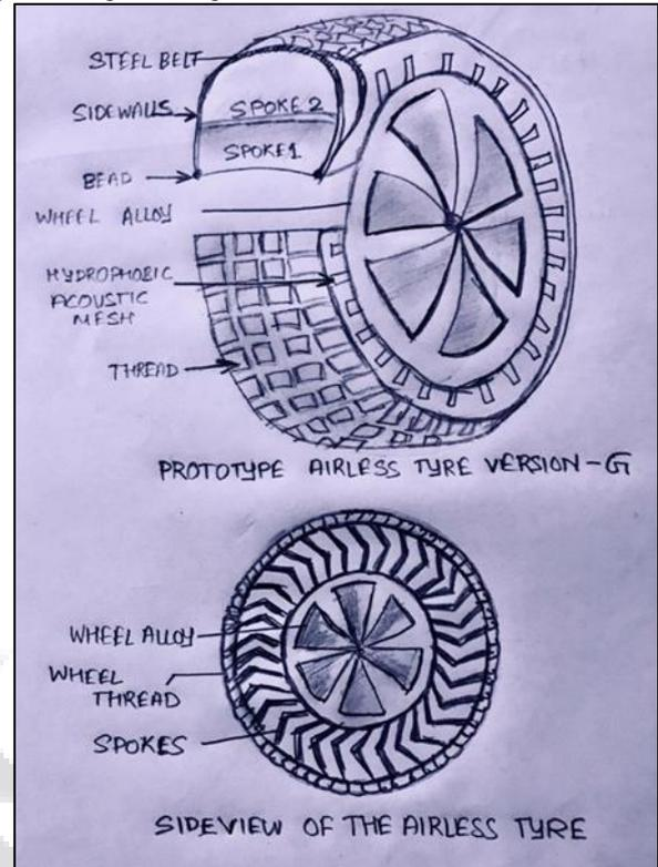
Fig. 8: Airless Tire (Version-G) Prototype Design
