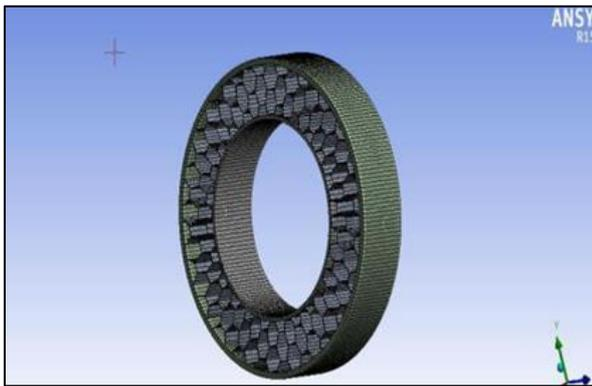
Fig. 3: .Honeycomb Structure with Tetrahedral mesh
