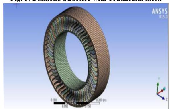
Fig. 6: Spoke type Structure with Tetrahedral mesh
