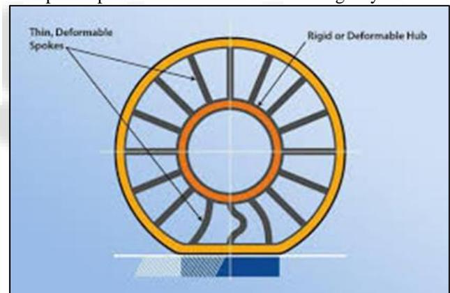
Fig. 2: Deformation in Airless Tire
