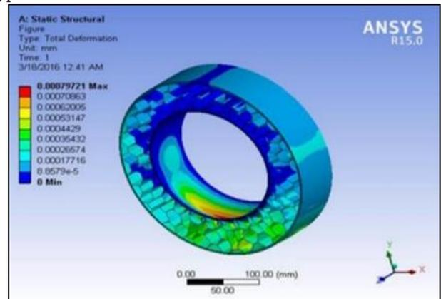
Fig. 7: Deflection of air less tire with Honey Comb Structure
