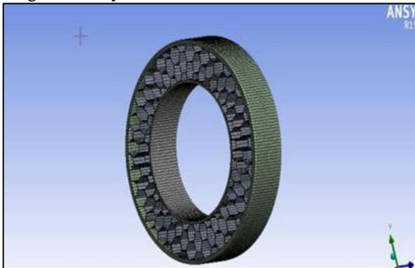
Fig. 4: .Triangular Structure with Tetrahedral mesh
