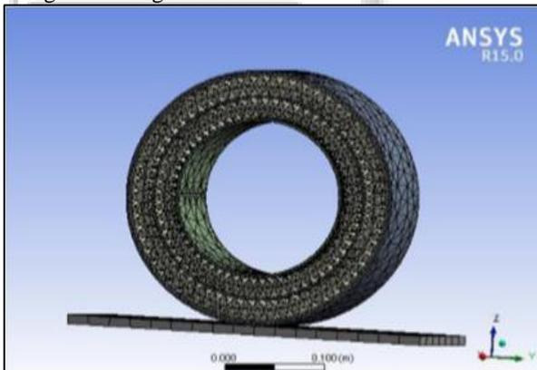
Fig. 5: Diamond Structure with Tetrahedral mesh
