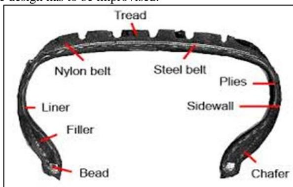
Fig. 1: Cut Section of a Conventional Tire
