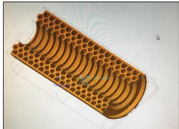
Fig. 10: 3-D Cut section of Airless tire (version-G)
