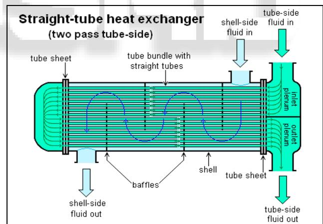
Fig. 1: straight tube heat exchanger (two pass tube)
