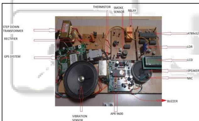
Fig. 6: a) Typical prototype model of the proposed system
