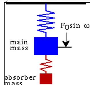
Fig. 2: The undamped dynamic vibration absorber.
