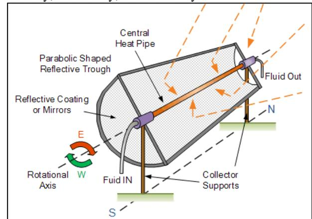
Fig. 1: Solar Parabolic Trough Collector
