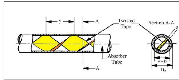
Fig. 2: Schematic representation of the twisted tape insert
