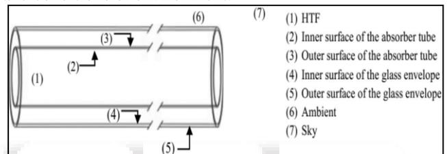
Fig. 3: Schematic of a fragment of HCE
