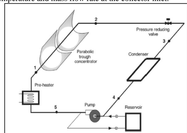
Fig. 4: Parabolic trough systems with pre-heater
