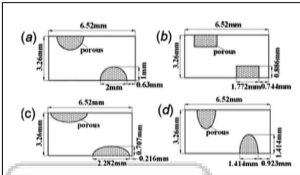
Fig. 3: Different forms of porous pin fin cross-section
