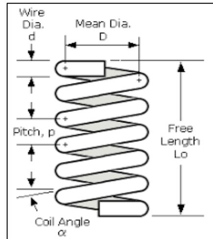
Fig. 1: Helical Coil Springs
