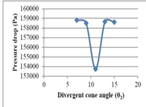
Fig. 7: Effect of divergent cone angle on pressure drop
