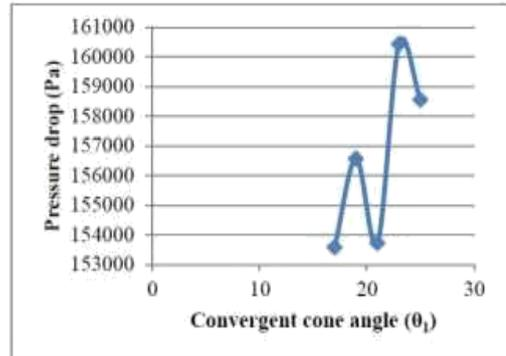
Fig. 6: Effect of convergent cone angle on pressure drop
