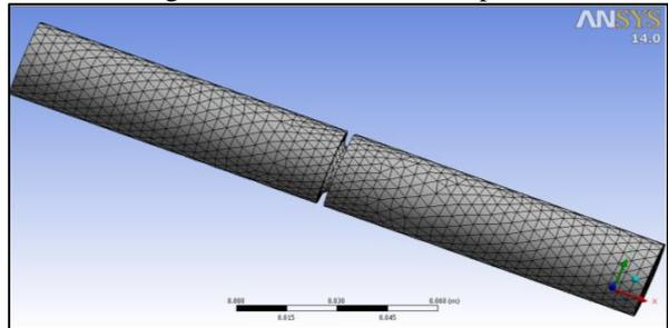
Fig. 9: Meshing of the model
