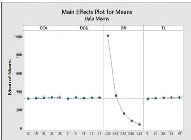
Fig. 5: Effects of Geometrical Parameters on Pressure Drop
