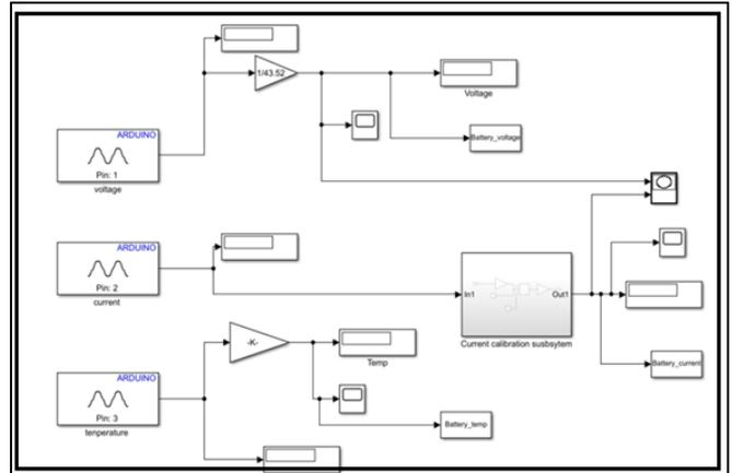
Fig. 4: MATLAB simulation model for battery parameter measurement
