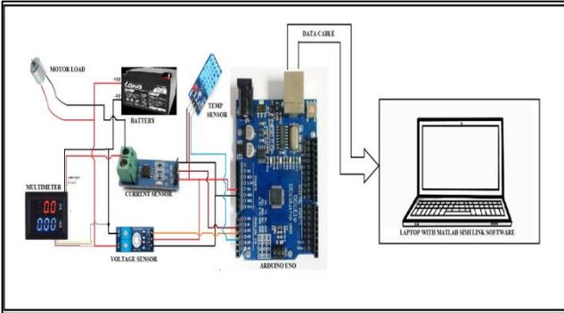
Fig. 2: Connection diagram of hardware components
