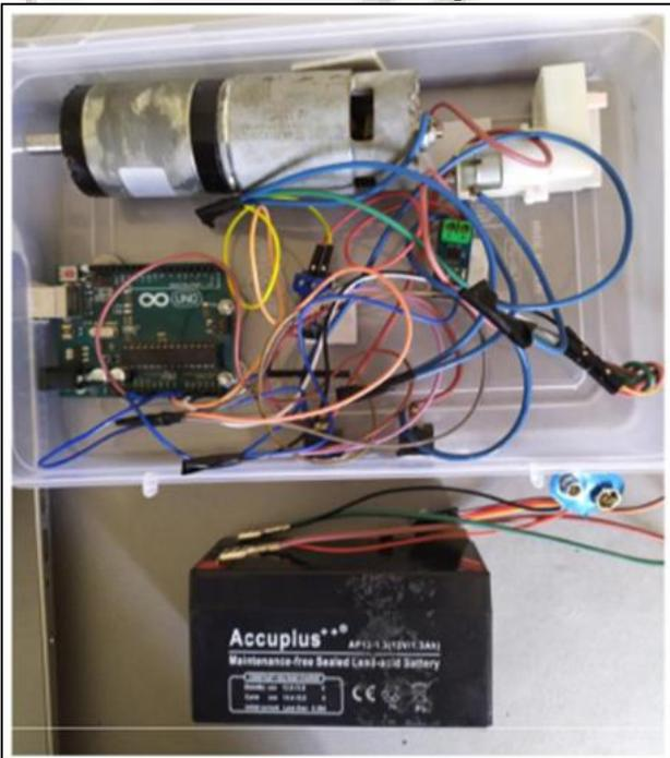
Fig. 3: Hardware implementation of proposed battery measurement system
