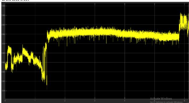
Figure 7 shows the real time battery body temperature versus time of operation of battery in which it observed that body temperature of battery directly depends upon battery load current. As load current increase then battery body temperature also increases. Initially battery temperature is around 29 Degree Celsius while at end battery temperature increases at maximum 29.9 Degree Celsius.
