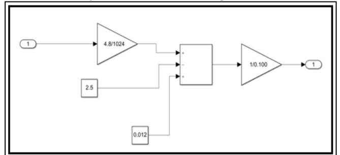
Fig. 5: MATLAB Simulink model of Current Calibration Subsystem
