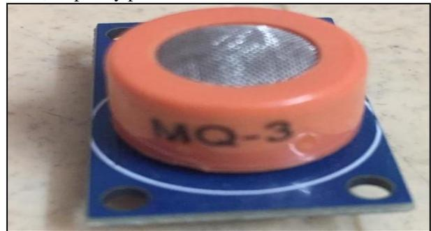
Fig. 1: Alcohol sensor
