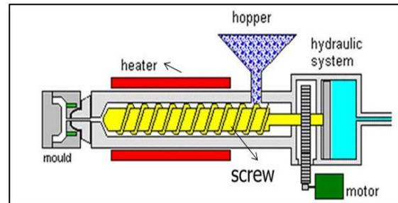
Fig. 1: Injection molding machine
