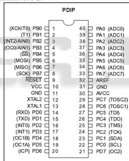
Fig 2: ATMEGA16 Pin Out
