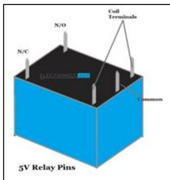
Fig. 3: Relay pin out
