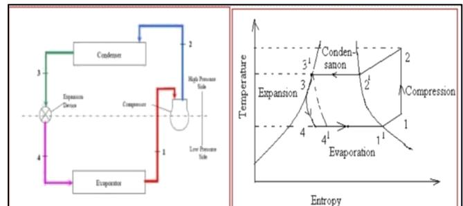
Fig. 1 Simple Vapour Compression system
