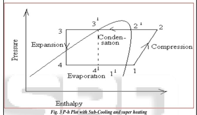
Fig. 3 P-h Plot with Sub-Cooling and super heating
