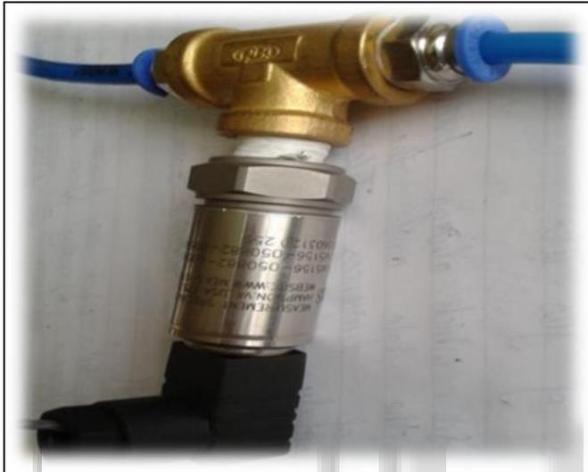
Fig. 5: Pressure Sensor
