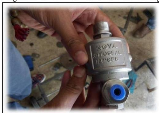
Fig. 4: Rotary Joint
