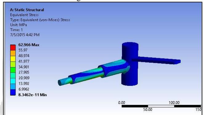
Fig. 6: Equivalent stresses
