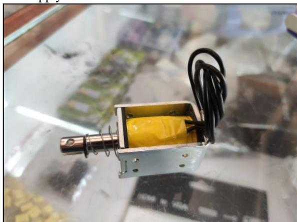
Fig. 5: Solenoid switch
