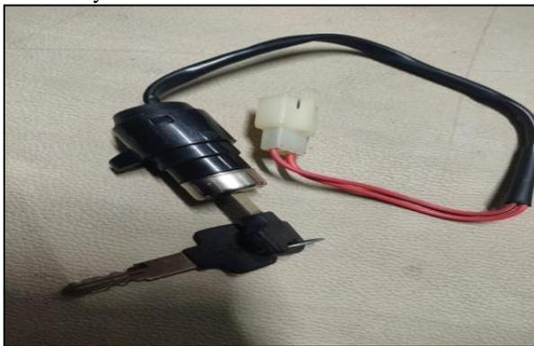
Fig. 4: Ignition ON OFF switch
