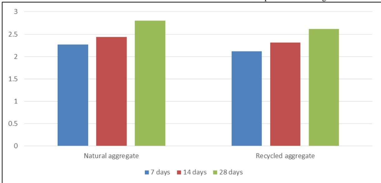
Fig. 2: Graphical representation of Split Tensile Strength of Concrete
