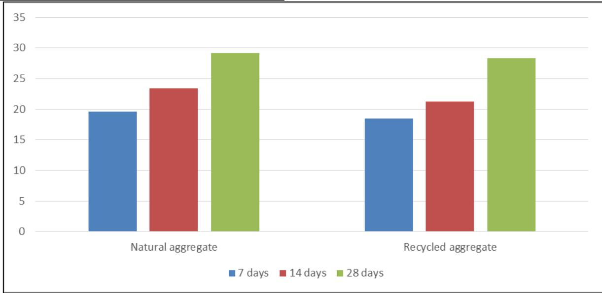
Fig. 1: Graphical representation of Compressive Strength of Concrete
