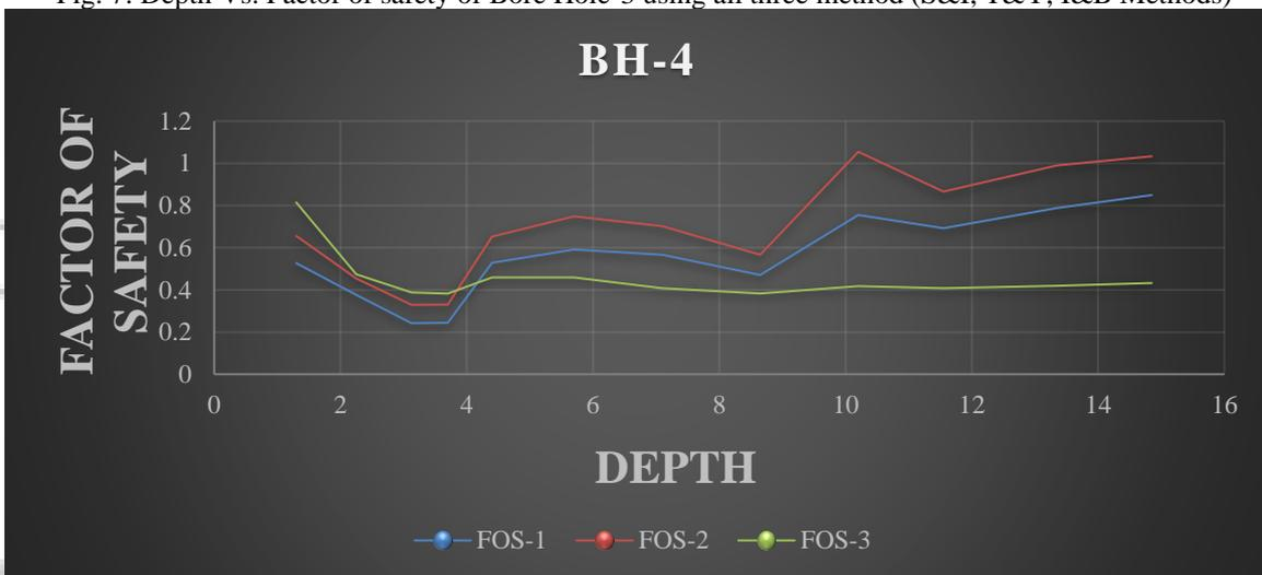
Fig. 8: Depth Vs. Factor of safety of Bore Hole-4 using all three method (S&I, T&Y, I&B Methods)
