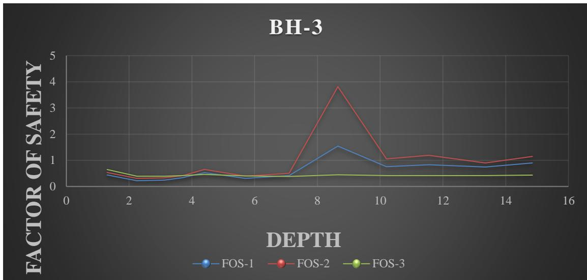
Fig. 7: Depth Vs. Factor of safety of Bore Hole-3 using all three method (S&I, T&Y, I&B Methods)
