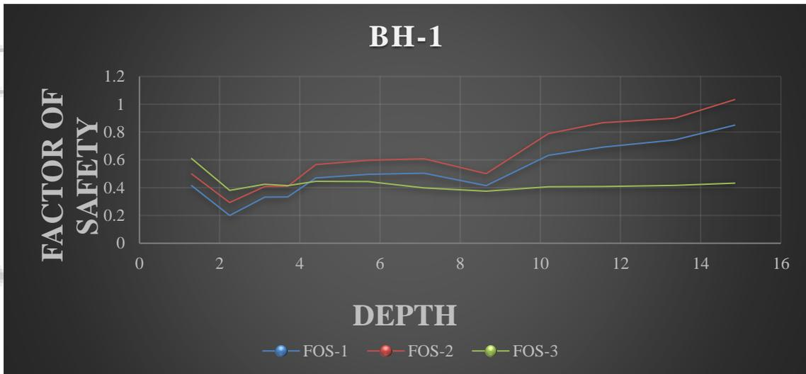
Fig. 5: Depth Vs. Factor of safety of Bore Hole-1 using all three method (S&I, T&Y, I&B Methods)
