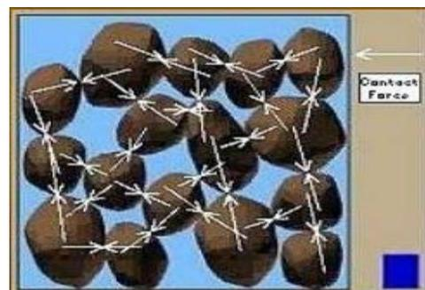
Fig. 3: Soil before liquefaction
