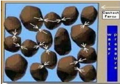
Fig. 4: Soil after liquefaction
