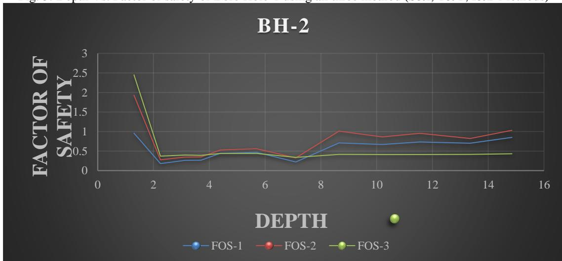
Fig. 6: Depth Vs. Factor of safety of Bore Hole-2 using all three method (S&I, T&Y, I&B Methods)
