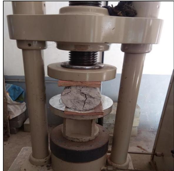
Fig. 8.2: Split tensile strength test on SFRC specimen
