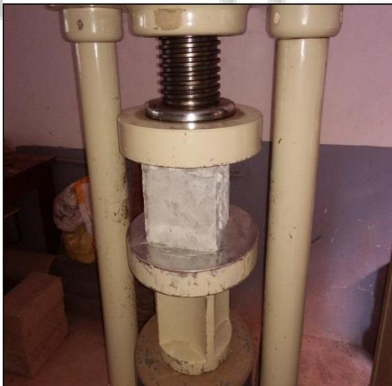
Fig. 8.1: Compression testing machine with sample
