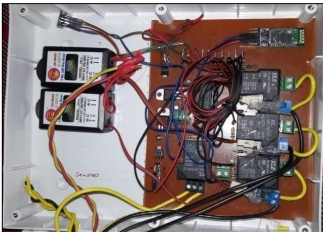
Fig. 2: Hardware setup with manual mode
