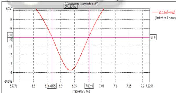
Fig. 15: Bandwidth of designed microstrip patch antenna for center frequency 6.93 GHz
