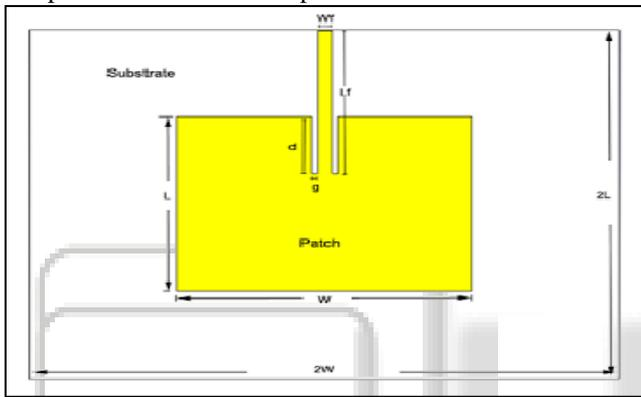
Fig. 4: Dimensions of an inset feed microstrip patch antenna
