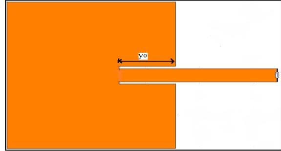
Fig. 5: An inset feed microstrip patch antenna
