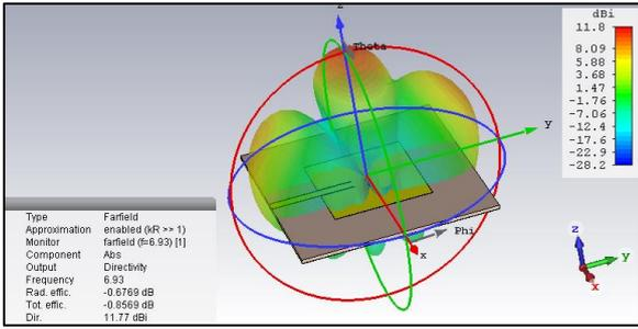
Fig. 20: 3 D radiation pattern of designed antenna at frequency 6.93 GHz
