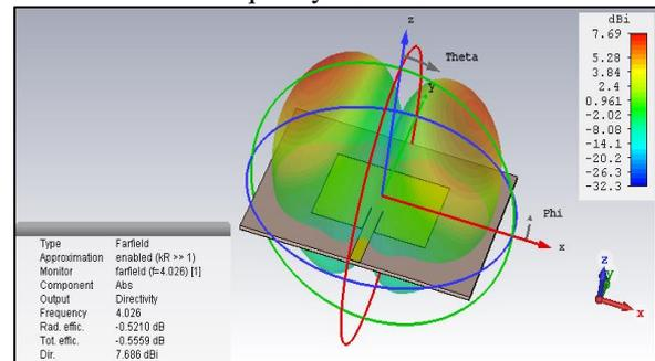
Fig. 18: 3 D radiation pattern of designed antenna at frequency 4.026 GHz
