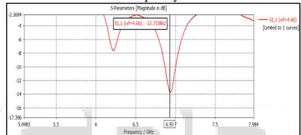
Fig. 10: Return loss of the designed microstrip patch antenna resonant at frequency 6.93 GHz
