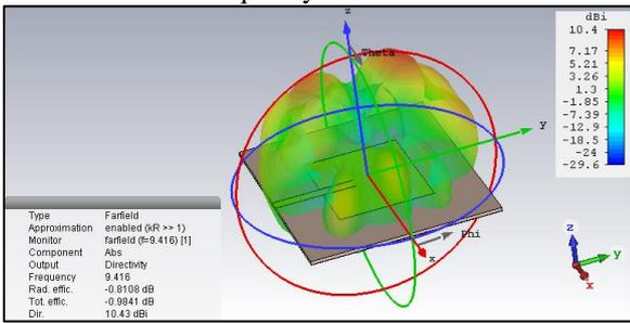
Fig. 21: 3 D radiation pattern of designed antenna at frequency 9.416 GHz
