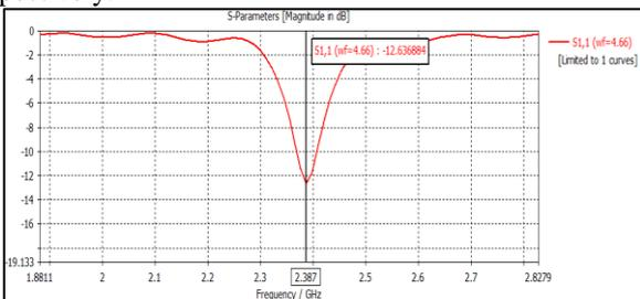
Fig. 7: Return loss of the designed microstrip patch antenna resonant at frequency 2.387 GHz
