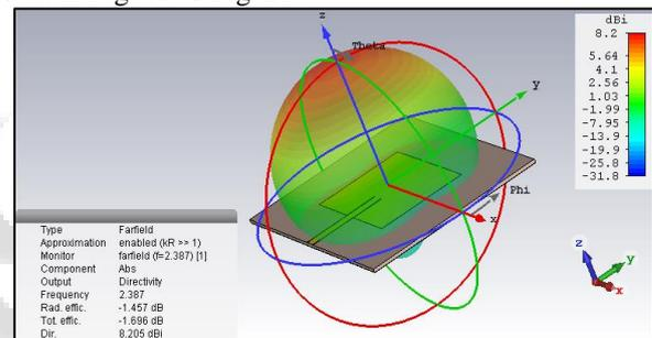
Fig. 17: 3 D radiation pattern of designed antenna at frequency 2.387 GHz
