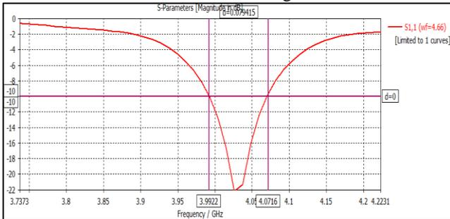
Fig. 13: Bandwidth of designed microstrip patch antenna for center frequency 4.026 GHz
