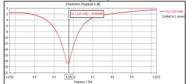
Fig. 9: Return loss of the designed microstrip patch antenna resonant at frequency 4.576 GHz
