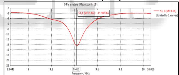
Fig. 11: Return loss of the designed microstrip patch antenna resonant at frequency 9.416 GHz
