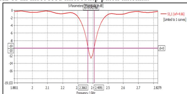
Fig. 12: Bandwidth of designed microstrip patch antenna for center frequency 2.387 GHz
