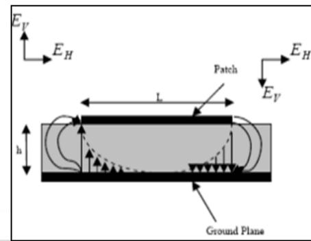
Fig. 3: Side view of microstrip patch antenna
