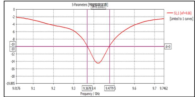
Fig. 16: Bandwidth of designed microstrip patch antenna for center frequency 9.416 GHz
