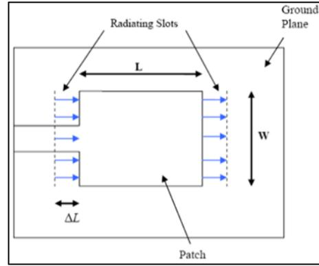
Fig. 2: Top view of microstrip patch antenna
