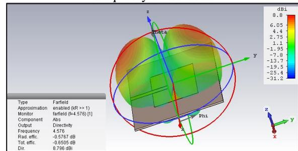
Fig. 19: 3 D radiation pattern of designed antenna at frequency 4.576 GHz
