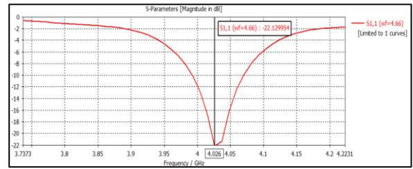
Fig. 8: Return loss of the designed microstrip patch antenna resonant at frequency 4.026 GHz
