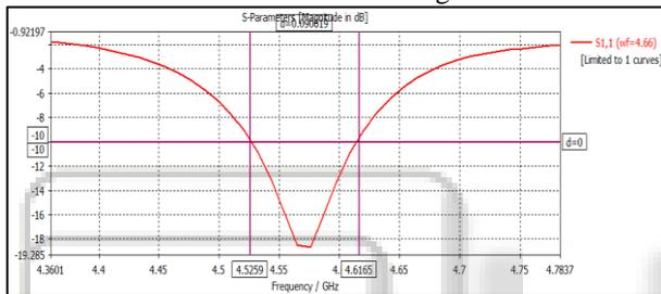
Fig. 14: Bandwidth of designed microstrip patch antenna for center frequency 4.576 GHz
