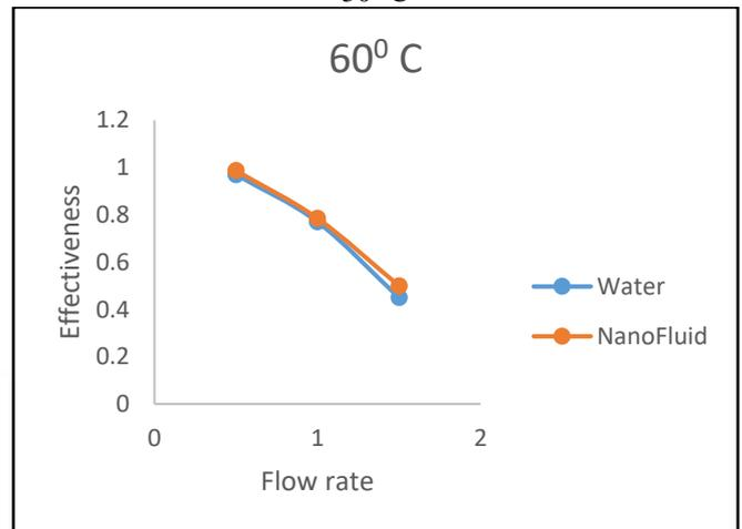
Fig. 1.12: Counter and Shell and Tube Heat Exchanger at 60<sup>0</sup> C
