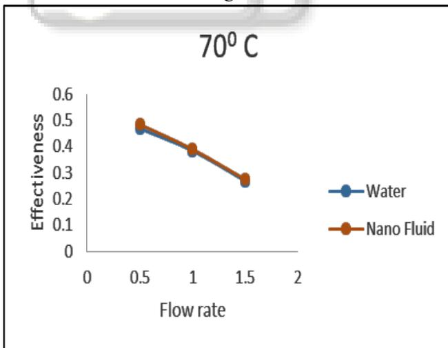
Fig. 1.10: Parallel and Shell and Tube Heat Exchanger at 70<sup>0</sup> C
