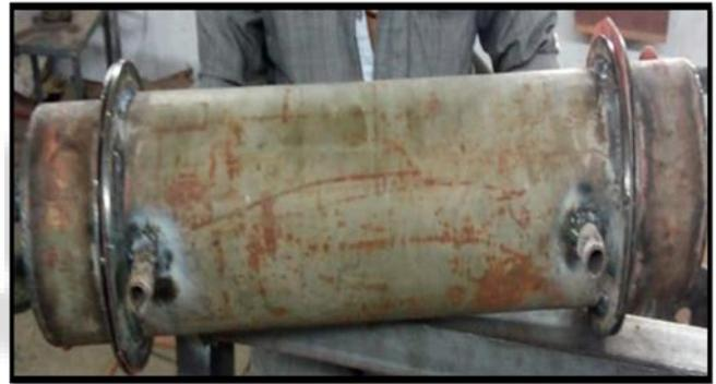
Fig. 1.7: Shell and tube Heat exchanger
