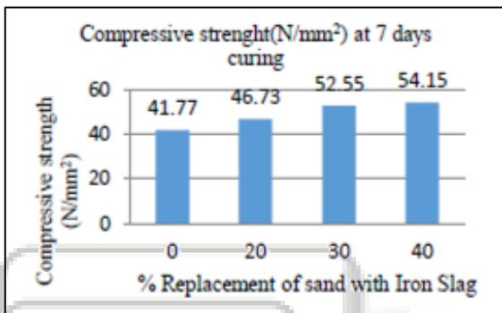
Fig. 7: Compressive Strength at 7 days
