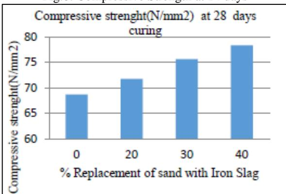
Fig. 9: Compressive Strength at 28 days
