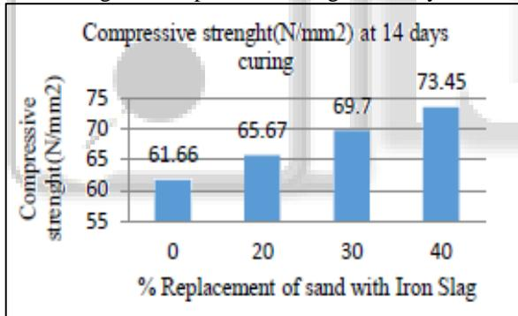
Fig.8: Compressive Strength at 14 days
