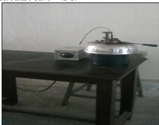
Fig. 8.3: Flash and Fire point Test Apparatus
