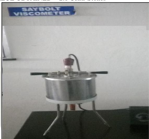
Fig. 8.2: Saybolt Viscometer
