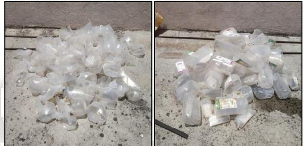
Fig. 7.2: Samples of Shredded Plastic Waste Saline Bottles
