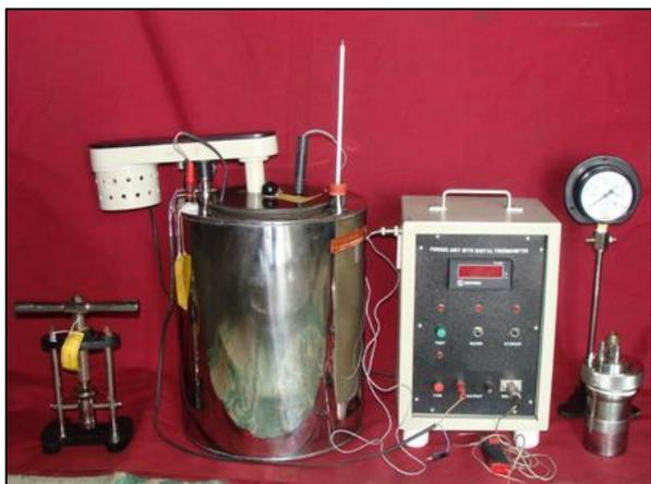
Fig. 8.1: Bomb Calorimeter
