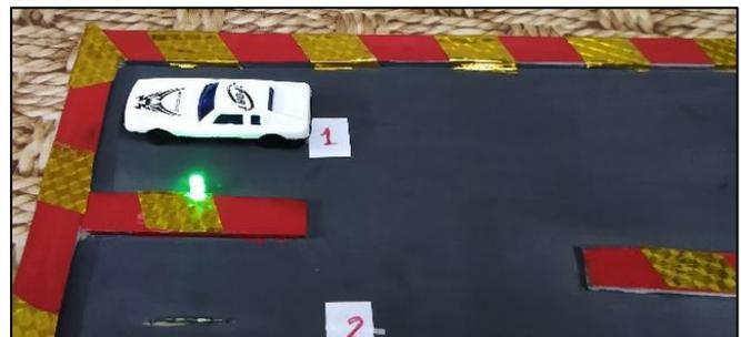
Fig. 8: Parking Slot with LED Indication
