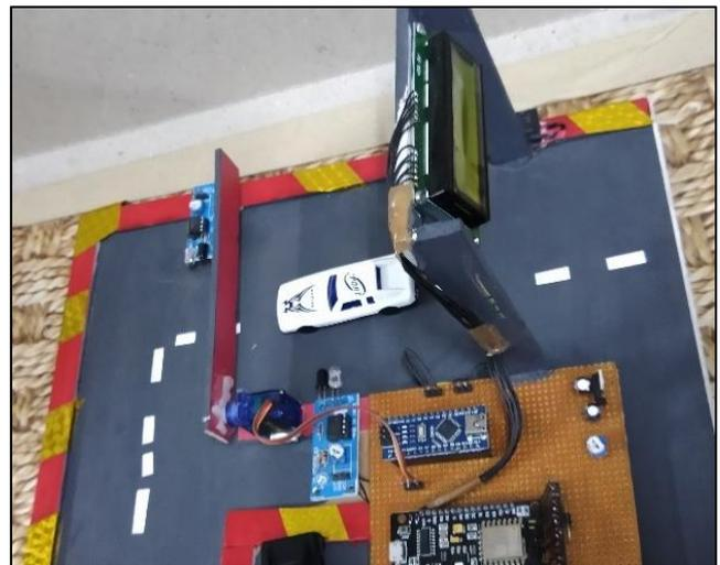
Fig. 6: Servo Motor Gate
