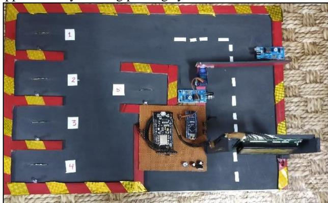
Fig. 10: Automated Car Parking System Model
