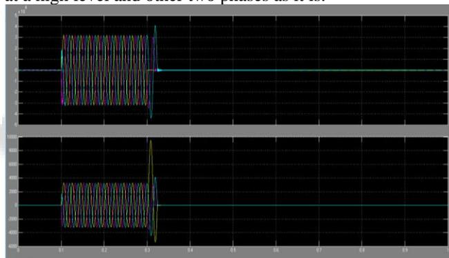
Fig. 12: Three phase of voltage and current signal at single phase to ground fault
