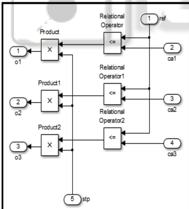
Fig. 5: Subsystem 1 for trip signal generation
