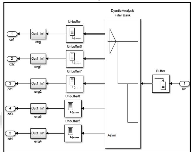
Fig. 3: Wavelet transform subsystem block in simulated model
