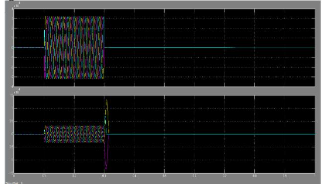
Fig. 17: Three phase of voltage and current signal at three phase to ground fault
