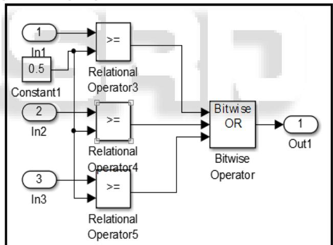
Fig. 6: OR gate subsystem
