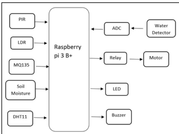
Fig. 2: Block Diagram of WSAN Based Smart Agriculture Monitoring System.
