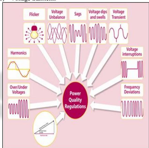
This figure shows the various issues with the power quality. These two figures are clearly shows the power quality issue has been seen in a system.
