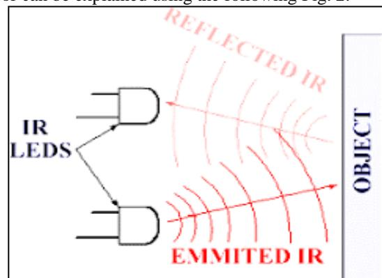
Fig. 2: principle working of an IR Sensor
