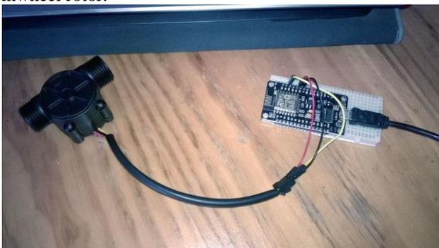
Fig. 5: Flow sensor Interfacing
