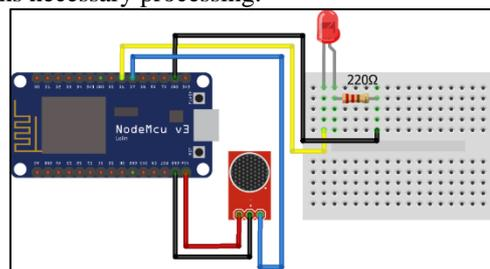
Fig. 4: Noise Sensor Interfacing
