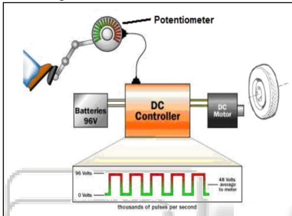
Fig. 2: Parts of an electric vehicle.
