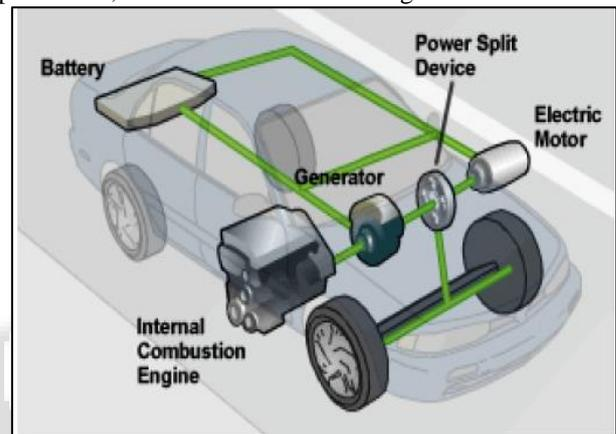
Fig. 3: Parts of a hybrid vehicle [4].
