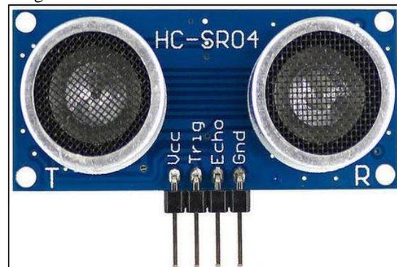
Fig. 3: Ultrasonic Sensor (HC-SR04)
