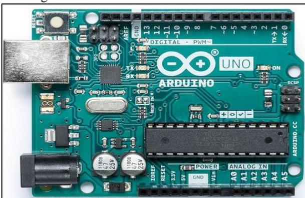
Fig. 2: Arduino Board <sup>[2]</sup>
