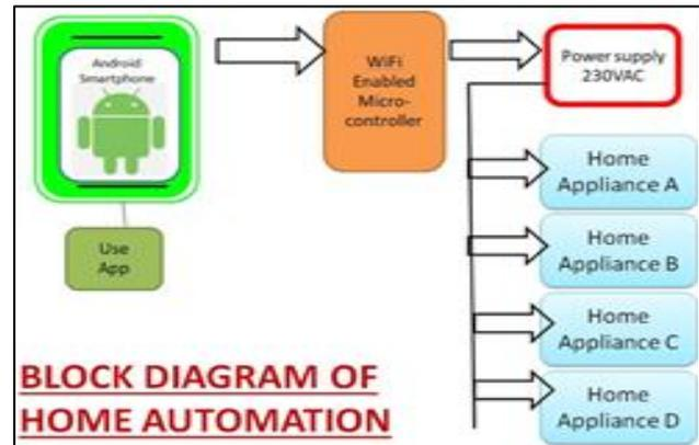
Fig. 1: Block Diagram of Home Automation
