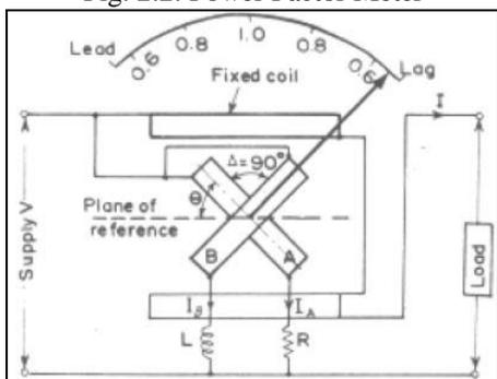
Fig. 2.3: Construction Diagram of PF Meter.
