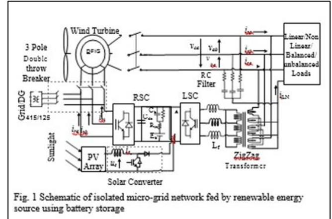
Fig. 1 Schematic of isolated micro-grid network fed by renewable energy source using battery storage
