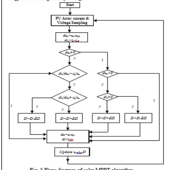
Fig. 3 Flow-diagram of solar MPPT algorithm
