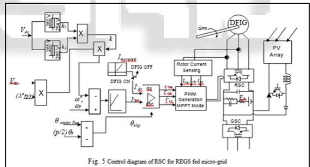
Fig. 5 Control diagram of RSC for REGS fed micro-grid
