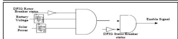
Fig. 6 Logic diagram for battery charging mode selection.
