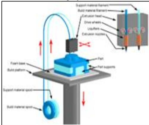
Fig. 2: Schematic Diagram of the FDM Process
