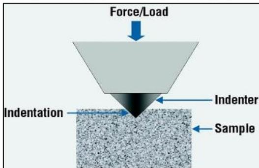
Fig. 8: Schematic Diagram of Rockwell Hardness
