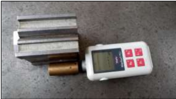
Fig. 3: Mar Surf PS1 Surface Roughness Tester
