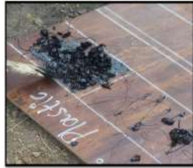
Fig. 6: Lay the prepared mixture on surface
