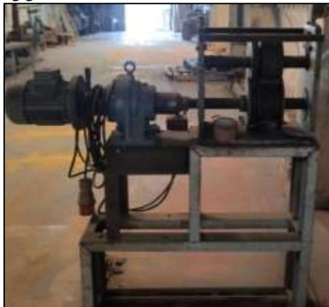
Fig. 3: Metal Foil Crimping Machine
