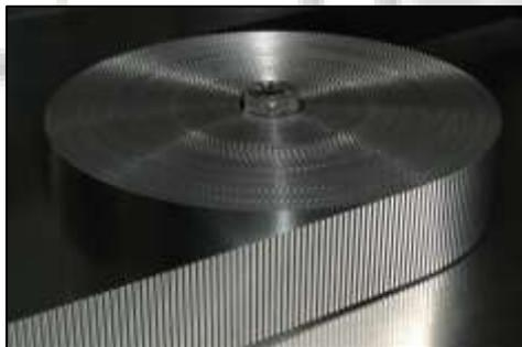
Fig. 8: Crimped Foil
