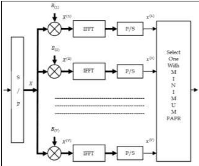
Fig. 1: Block diagram of OFDM system with Selective Mapping (Han & Lee, 2005)
