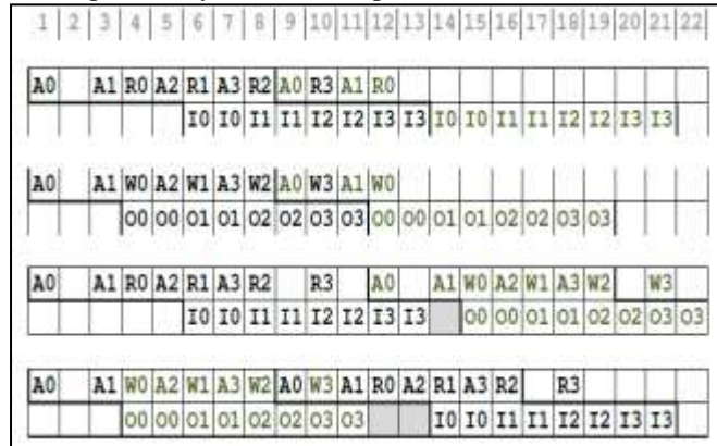
Fig. 3: Eight word operations interleaved over four banks
