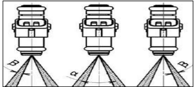
Fig. 3: Schematic diagram of spray cone angles: left beta angle (left), alpha angle (middle) and right beta angle (right).
