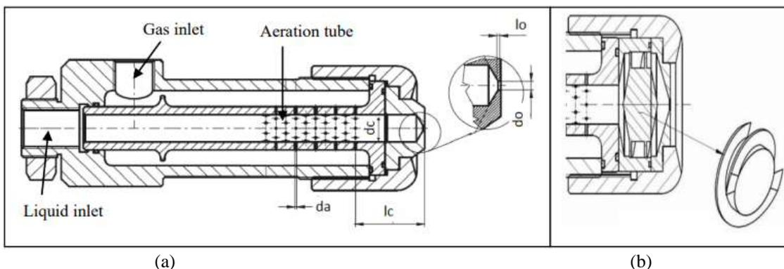
Fig. 2: Injector internal geometries (a) Full body without swirler (b) with Swirler
