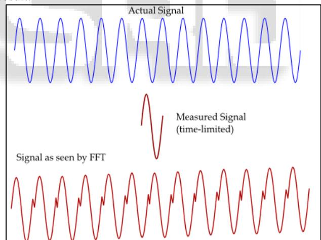
The F.F.T protocol assumes that the received signal are present an infinite duration. This result is based on the presumption that the wave signal acquired in the time record itself and again. If at the beginning and the end of the time record, the amplitude of the original signal is non zero, the FFT will measure a result at each compilation interval for a waveform with sharp edges. The sample of a simple sine wave signal will demonstrate this effect.
