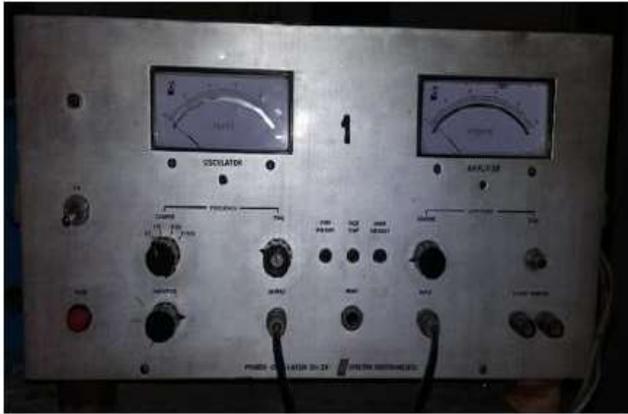
Fig. 3: Power Amplifier cum Signal Generator
