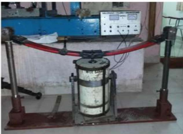
Fig. 4: Electrodynamic Vibration Shaker System with Vibration Table and Power Amplifier cum Signal Generator
