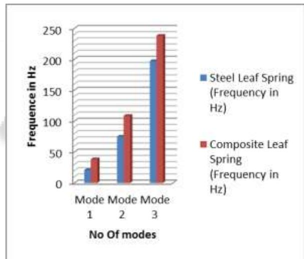
The schematic results of the static test using the impact hammer for standard steel leaf springs are shown below. As seen in Fig. the free vibration outcomes for Steel Leaf Spring are
