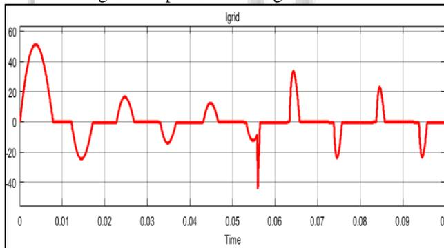
Fig. 3.10: Input Grid Current Waveform during Pre-charge Time
