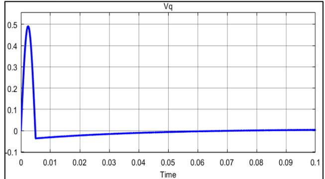
Fig. 3.5: Controlled Vq Generated from PLL
