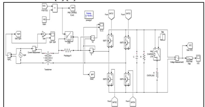
Fig. 2.1: Power Circuit of Active Front End Converter
