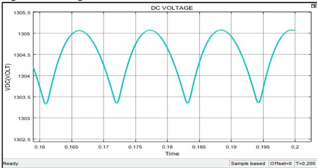
Fig. 3.2: Ripple Voltage of Diode Uncontrolled Rectifier
