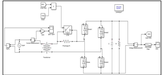
Fig. 1.1: Power Circuit of Diode Uncontrolled Rectifier
