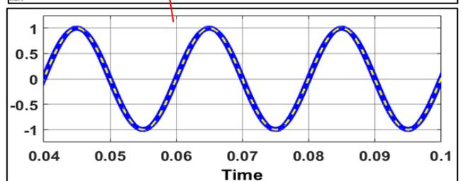
Fig. 3.7: Comparison of Sine Wave Generated from Theta(PLL) and Theta(REF)
