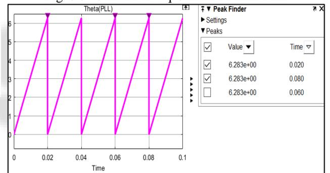
Fig. 3.6: Controlled Theta Generated from PLL
