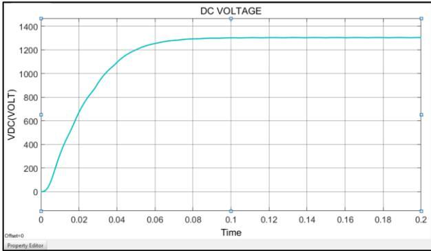
Fig. 3.1: Voltage Waveform of Diode Uncontrolled Rectifier
