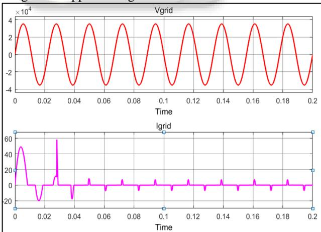
Fig. 3.3: Input Side Grid Voltage and Current Waveform of Diode Uncontrolled Rectifier
