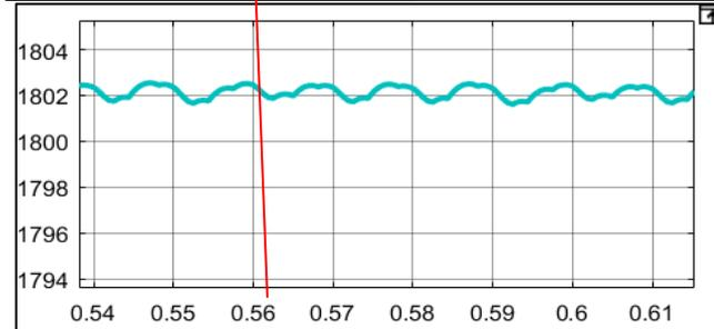
Fig. 3.8: Output DC Voltage Waveforms with SPWM Control
