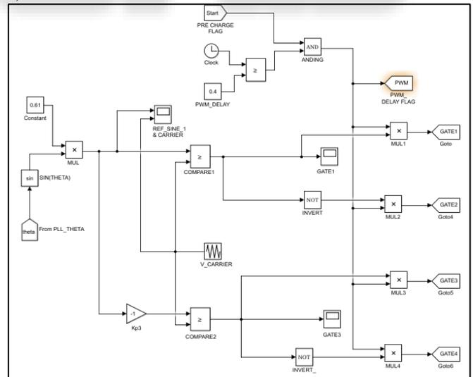
Fig. 2.3: SPWM Control Circuit
