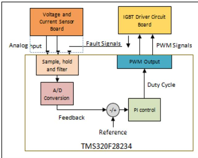
Fig. 4: BMS Controller Design
