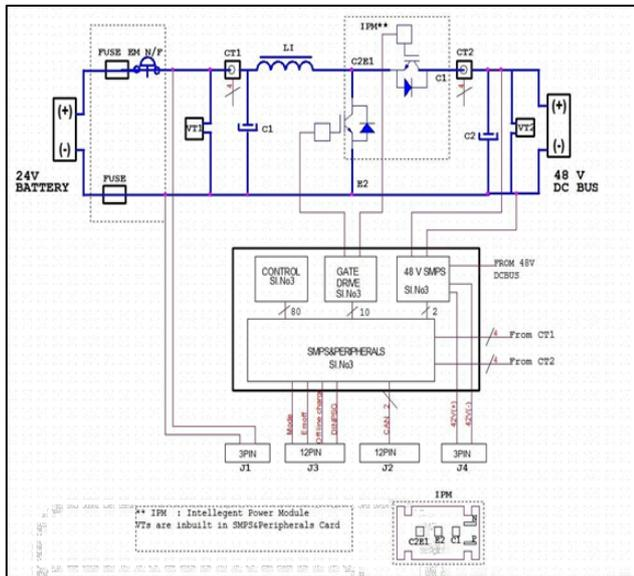
Fig. 2: Block Model of the BMS of DC Nanogrid
