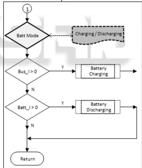
Fig. 5: Flowchart for BMS operation
