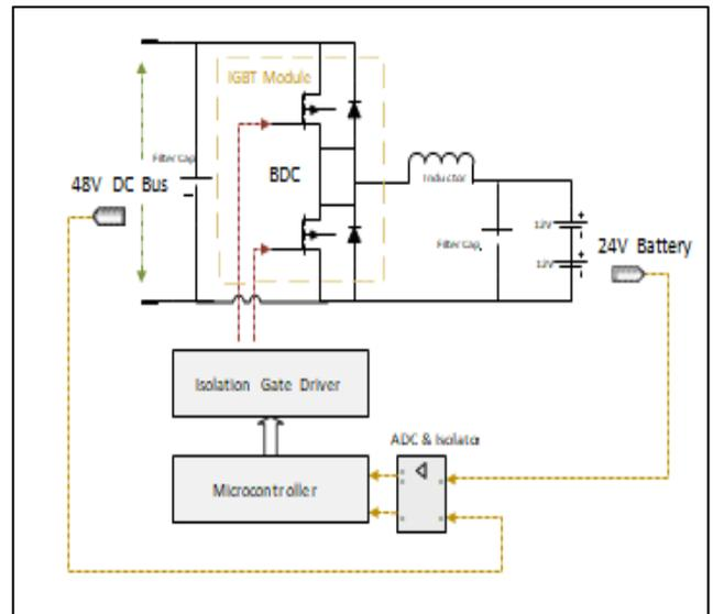
Fig. 3: BMS Power circuit topology
