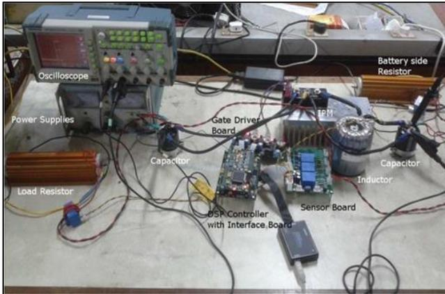
Fig. 6: BMS Hardware Setup
