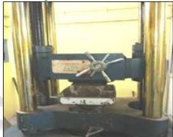
Fig. 3.2: Universal testing Machine
