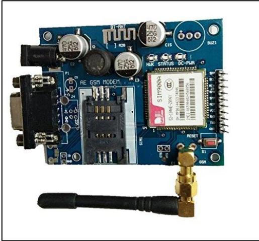
Examples of GSM modem which is used to sending SMS through GSM like temperature sensor or solid state relay .due to this practice the advantages of GSM is no need to waste time by doing the work manually and transportation of SMS or the means of call and medical services.
