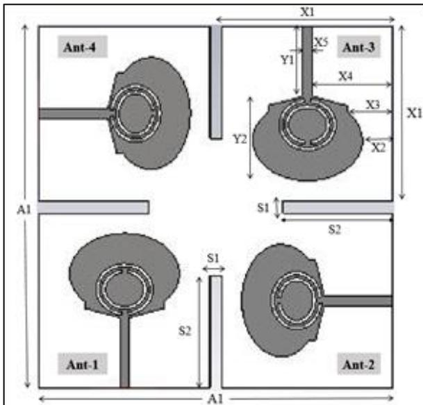
Fig. 2: Proposed design of Four port MIMO antenna
