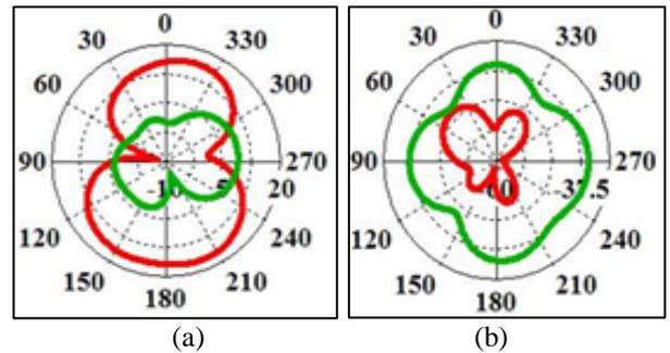
Fig. 9: Radiation Patterns of the Proposed antenna at 4.952 GHz with port 2 excitation (a) XZ-plane (b) YZ-plane
