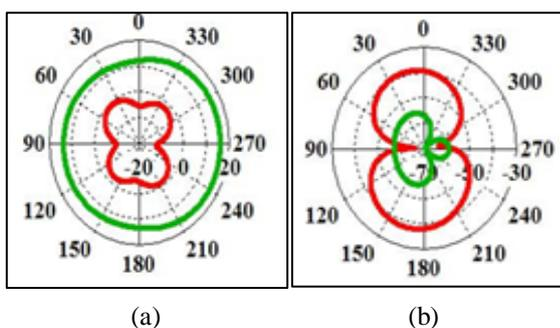
Fig. 8: Radiation Patterns of the Proposed antenna at 3.15 GHz with port 1 excitation (a) XZ-plane (b) YZ-plane
