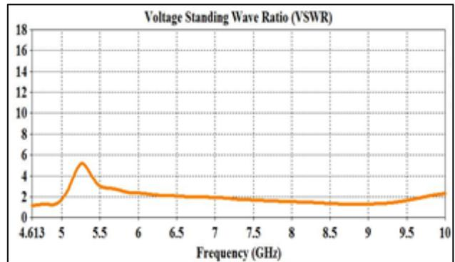
Fig. 4: VSWR of MIMO Antenna
