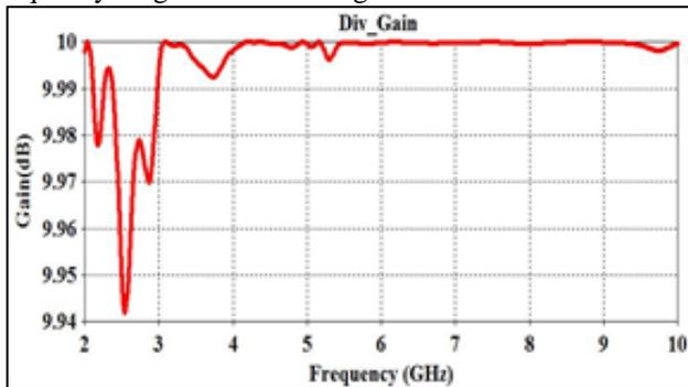
Fig. 7: Diversity Gain of MIMO antenna
