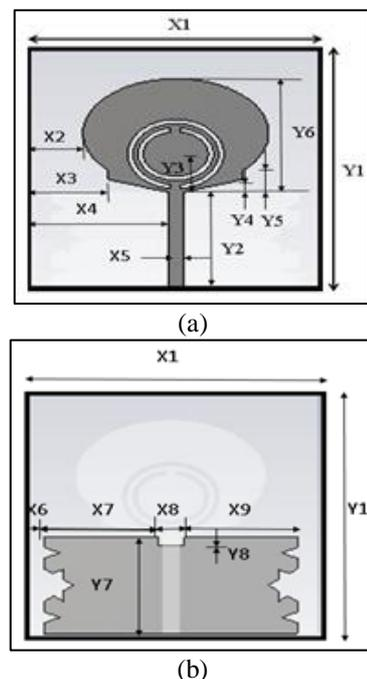
Fig. 1: Single antenna a) Front view b) Back View
