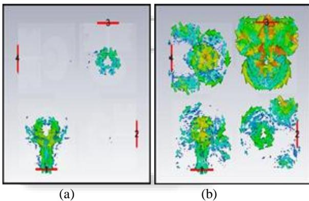
Fig. 7: Surface current distribution in proposed MIMO antenna (a) Port 1 excitation at 3.15 GHz (b) Port 3 excitation at 8.8452 GHz
