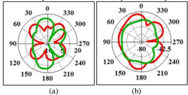
Fig. 10: Radiation Patterns of the Proposed antenna at 8.8492 GHz with port 3 excitation (a) XZ-plane (b) YZ-plane
