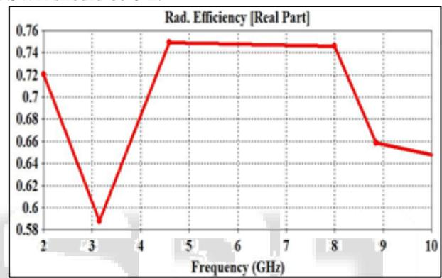
Fig. 5: Efficiency of MIMO Antenna
