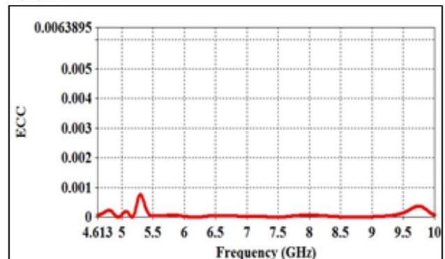
Fig. 6: ECC of MIMO antenna
